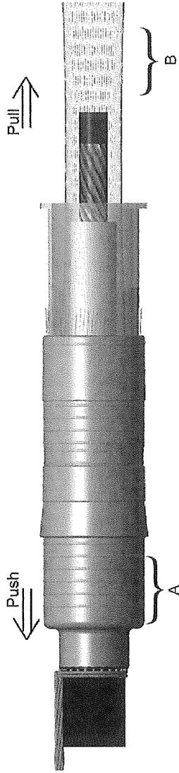
Push the silicone termination with one hand to move down on the cable (part A) while the other hand pulls on the red net (part B).
